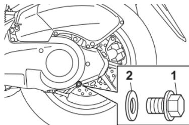
1. Final transmission oil drain bolt
