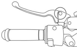
The pivoting points of the front and rear brake levers must be lubricated at the intervals specified in the periodic maintenance and lubrication chart.
