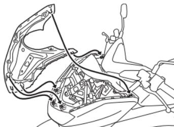
8. Install the windshield by installing the screws.
