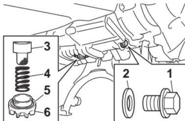
1. Engine oil drain bolt A
