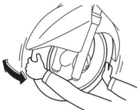
The front and rear wheel bearings must be checked at the intervals specified in the periodic maintenance and lubrication chart. If there is play in the wheel hub or if the wheel does not turn smoothly, have a Yamaha dealer check the wheel bearings.
