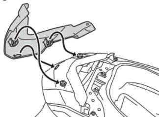
9. Install the grab bar by installing the bolts, and then tightening them to the specified torque.
