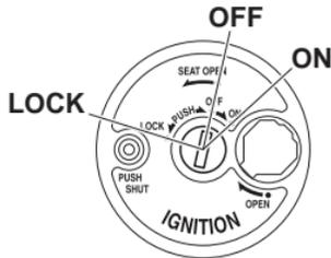
The main switch/steering lock controls the ignition and lighting systems, and is used to lock the steering. The various main switch positions are described below.
