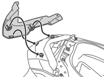
12. Install the grab bar by installing the bolts, and then tightening them to the specified torque.
