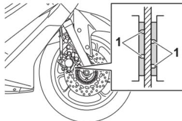
1. Brake pad wear indicator groove
